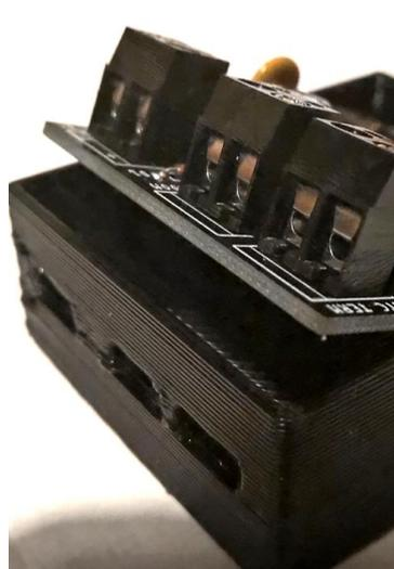
*Figure 3: Terminal Blocks Lifted From Case*
