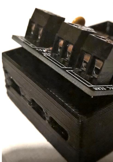
Figure 3: Terminal Blocks Lifted From Case
